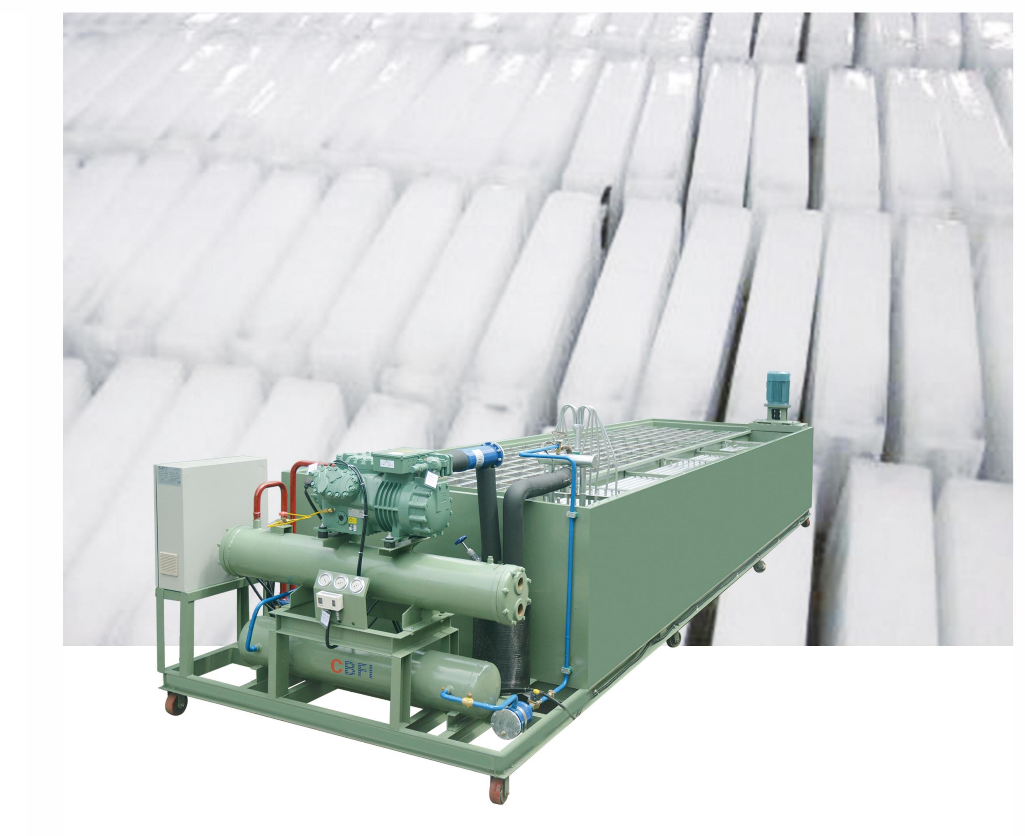
Guangzhou Icesource block ice machine capacity can be 1 ton to 200 tons. 1 tons of -10 tons adopt integrated design.
