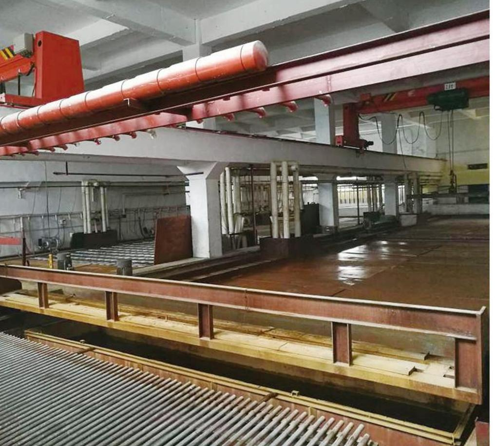
120 tons Civil Construction Block Ice Machine (Transparent ice)
